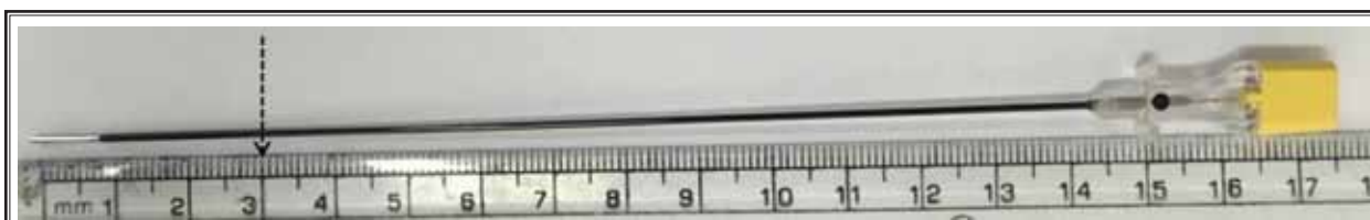
Fig. 2. A 150 mm RF needle with 10 mm active tip. Dotted arrow indicates the site of breach in the integrity of the insulating sheath.
